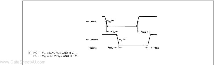
Fig.6 Waveforms showing the input (nA) to output (nY) propagation delays and the output transition times.
